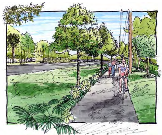
Proposed widening of existing sidewalk on west side of A1A to 10-foot multi-use trail with landscaped buffer - four lane section north of Fairfield Boulevard to Duval County line.
