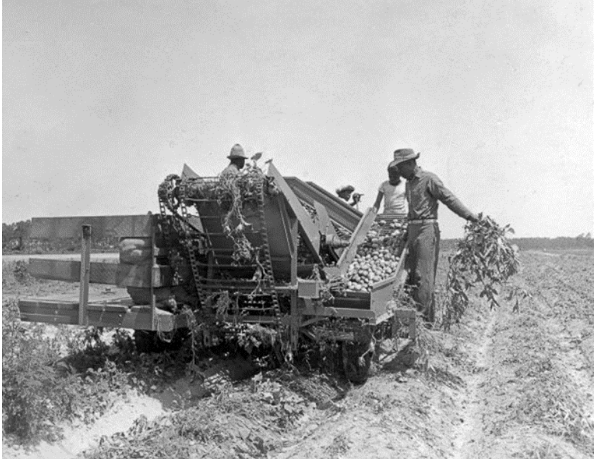
Figure 3-31. Workers using modernized equipment to harvest potato crops, ca. 1947; this was the second season for the Parrish-Middleton potato machine, the first machine patented for digging, sorting, and bagging potatoes in the field.; once implemented four men could do the work of a thirty-to-forty-man crew (image courtesy State Library and Archives of Florida, Florida Memory, Department of Commerce Collection, C006420).
