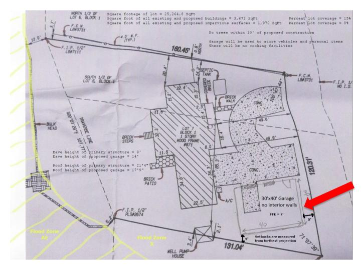
The above-proposed site plan, provided by the applicant and in its entirety, depicts the location and layout of the proposed detached garage. The full site plan is included in **Attachment 1 Supporting Documents.**
