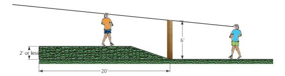
(2) If there is a grade change of more than two (2) feet within 20 feet of the of the boundary of the adjoining properties, and a fence is to be constructed at the lowest elevation of grade change, then a fence may be constructed to a maximum height of eight (8) feet.
