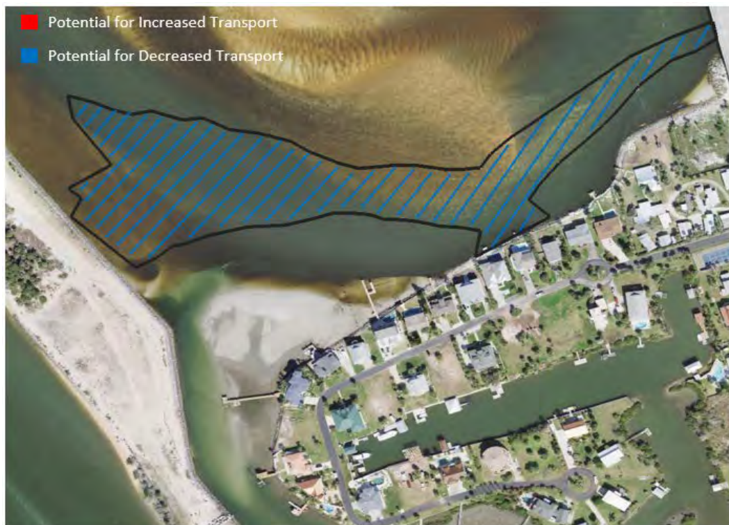
Figure 1.39 Scenario 4 (Dredged Inlet Channel) Effects on Erosion during Flood Flow
