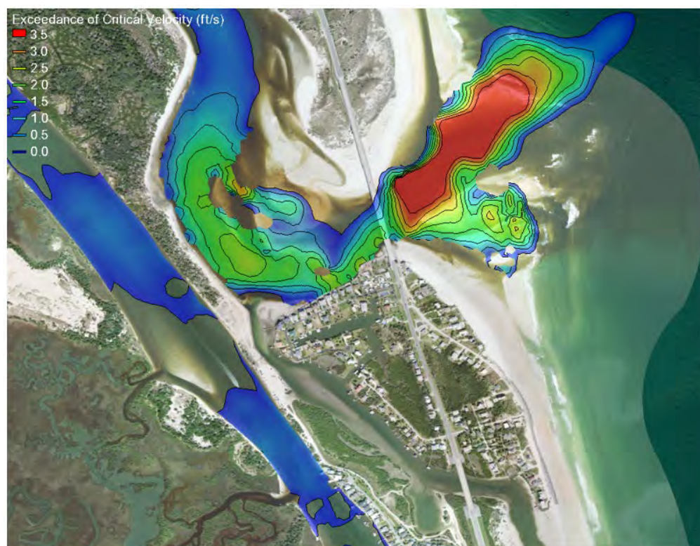
Figure 4.28 Exceedance of Critical Velocity at Peak Ebb Flow – Existing Conditions
