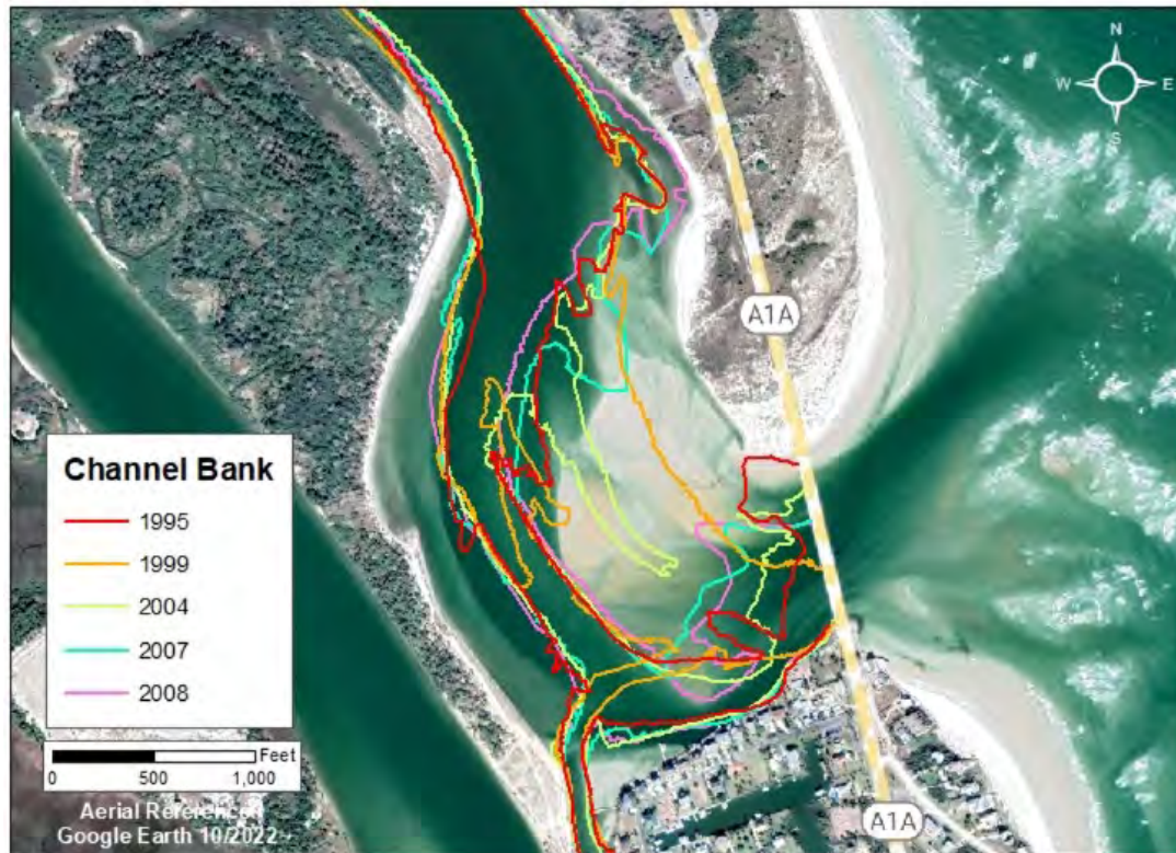
Figure 4.12 Matanzas Inlet Primary Channel Positions from 1995–2008
