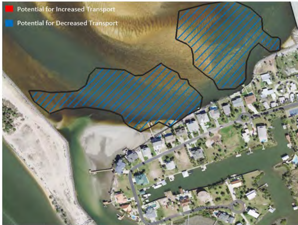
Figure 1.38 Scenario 4 (Dredged Inlet Channel) Effects on Erosion during Ebb Flow
