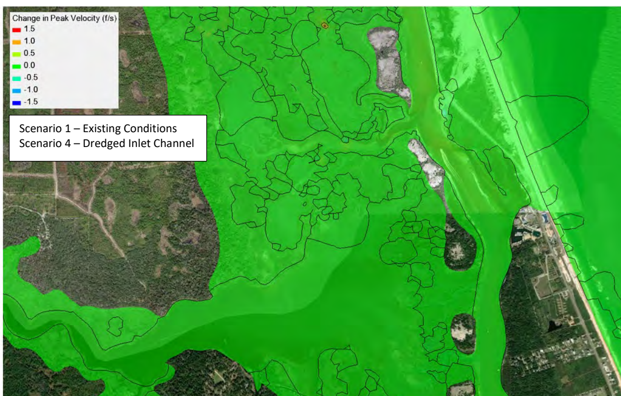
Figure 4.43 Change in Velocity within Inlet at Peak Ebb Flow — Scenario 4 vs. Existing Conditions
