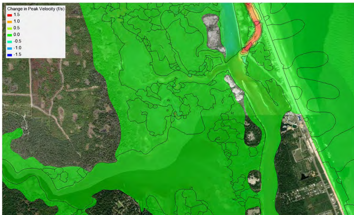
Figure 1.44 Change in Velocity within Inlet at Peak Ebb Flow – Scenario 3 vs. Existing Conditions
