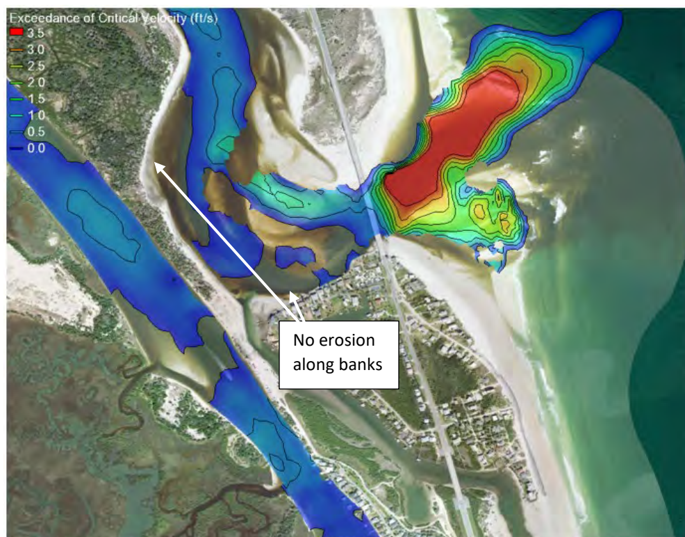
Figure 4.34 Exceedance of Critical Velocity at Peak Ebb Flow – Scenario 4 (Dredged Inlet Channel)
