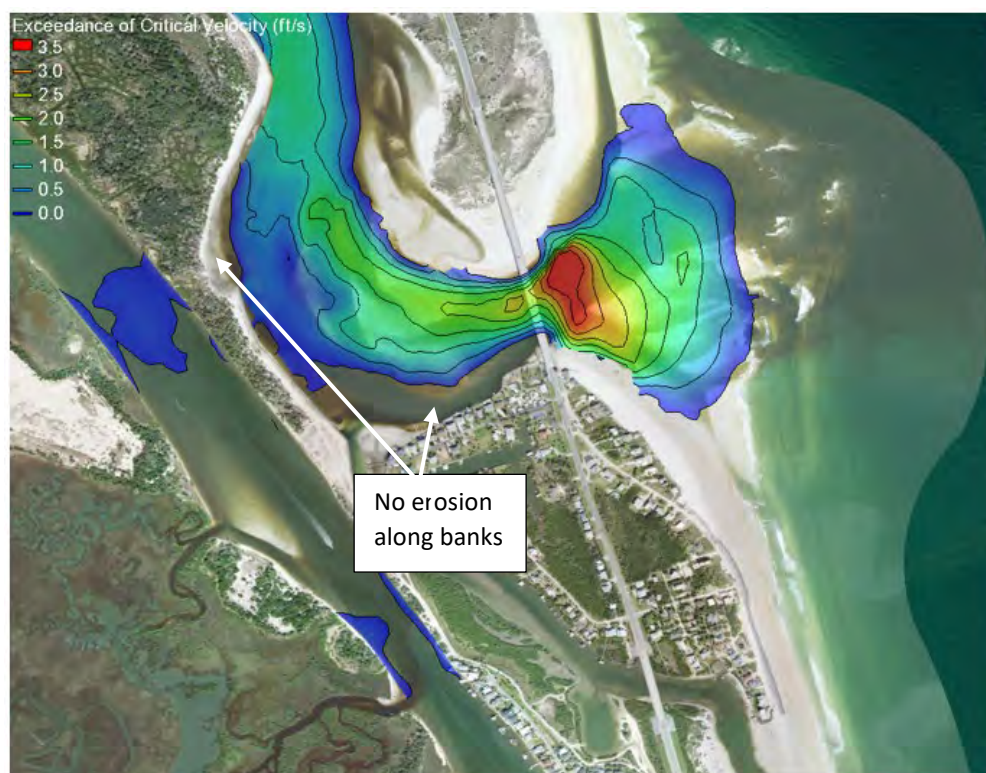
Figure 4.35 Exceedance of Critical Velocity at Peak Flood Flow – Scenario 4 (Dredged Inlet Channel)
