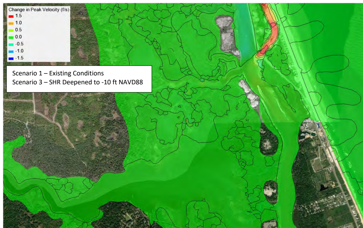
Figure 4.42 Change in Velocity within Inlet at Peak Ebb Flow – Scenario 3 vs. Existing Conditions
