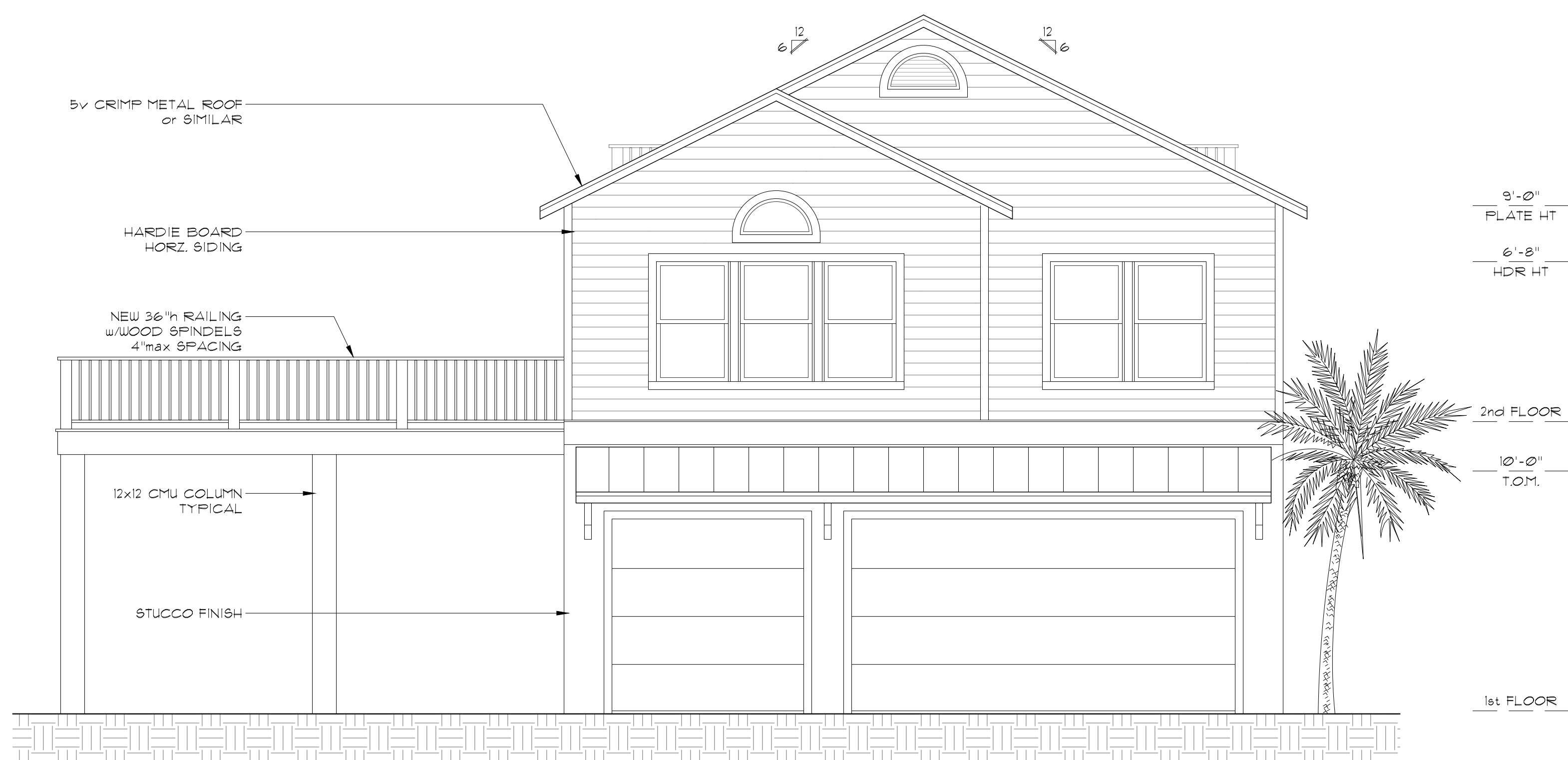
South Elevation 1/4"=1'-0" Garage
