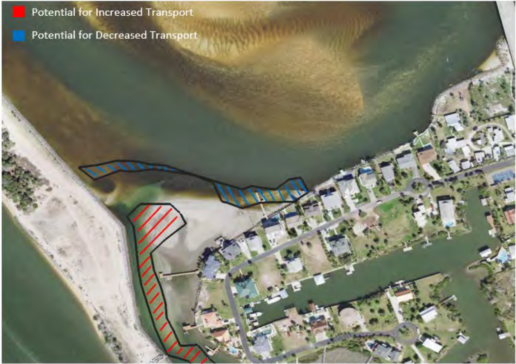
Figure 1.34 Scenario 2 (SHR Deepened to -6 ft NAVD 88) Effects on Erosion during Ebb Flow
