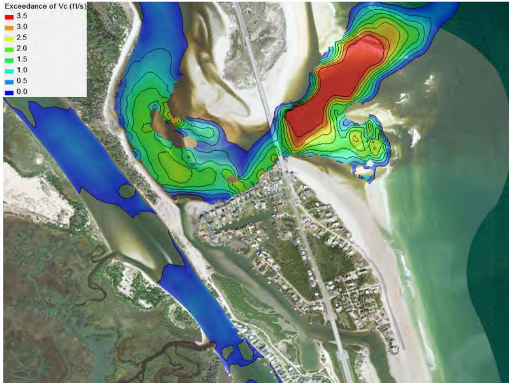
Figure 1.26 Exceedance of Critical Velocity at Peak Ebb Flow – Existing Conditions
