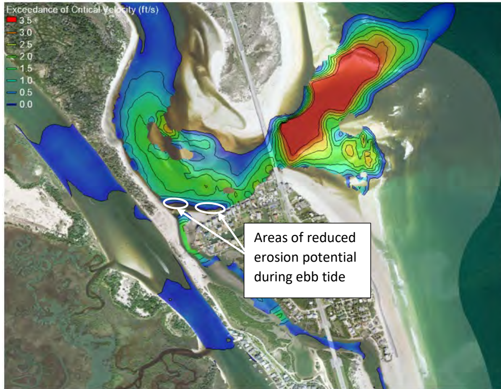
Figure 4.30 Exceedance of Critical Velocity at Peak Ebb Flow – Scenario 2 (SHR Deepened to -6 ft NAVD88)
