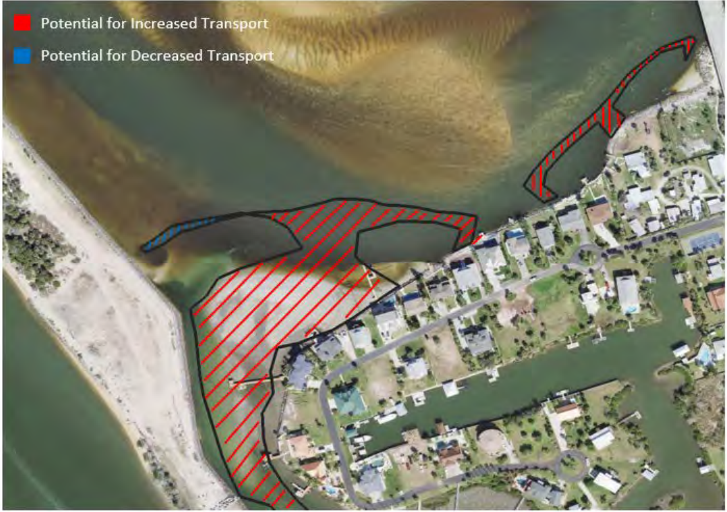
Figure 1.35 Scenario 2 (SHR Deepened to -6 ft NAVD 88) Effects on Erosion during Flood Flow
