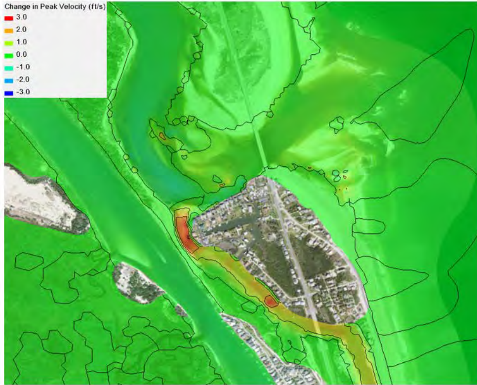
Figure 1.20 Change in Velocity within Inlet at Peak Ebb Flow – Scenario 3 vs. Existing Conditions
