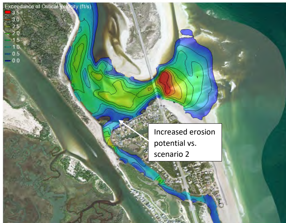
Figure 4.33 Exceedance of Critical Velocity at Peak Flood Flow – Scenario 3 (SHR Deepened to -10 ft NAVD88)
