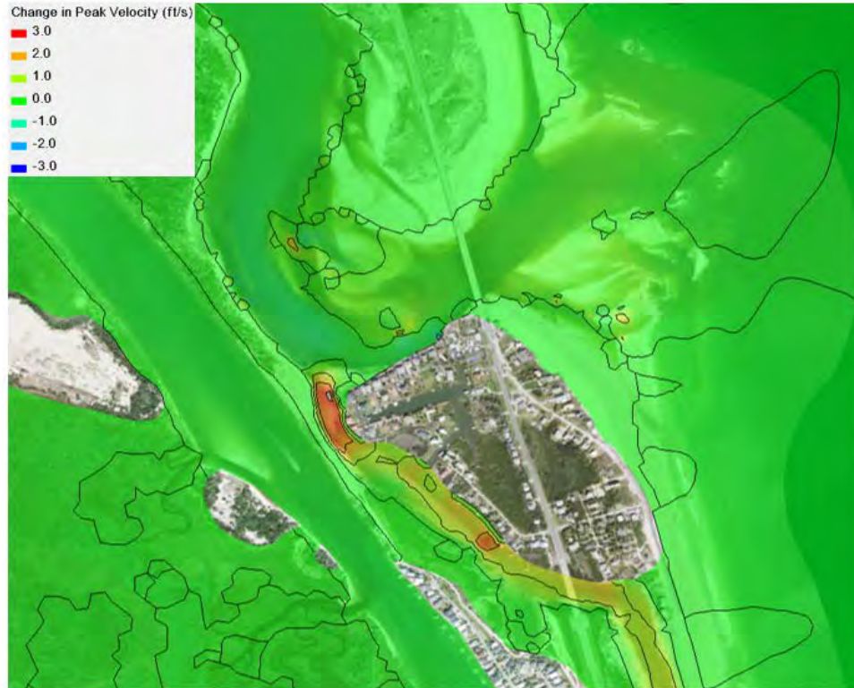
Figure 1.16 Change in Velocity within Inlet at Peak Ebb Flow – Scenario 2 vs. Existing Conditions
