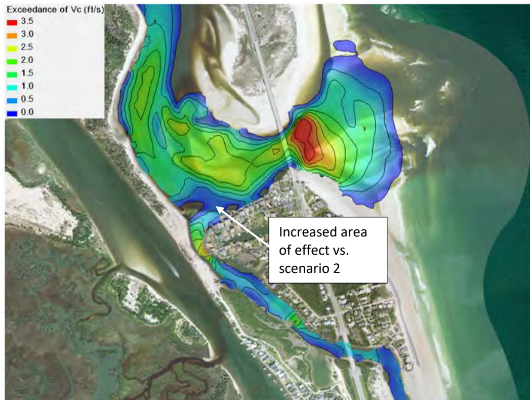
Figure 1.31 Exceedance of Critical Velocity at Peak Flood Flow – Scenario 3 (SHR at -10 ft NAVD 88)
