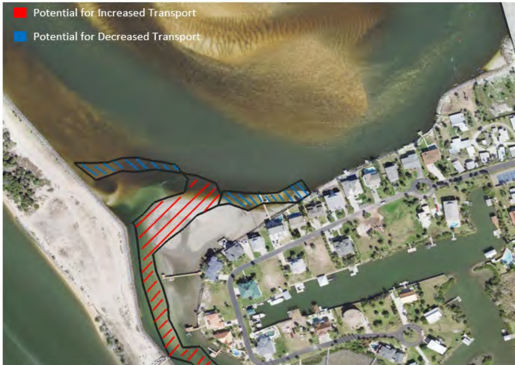
Figure 4.38 Scenario 3 (SHR Deepened to -10 ft NAVD88) Effects on Erosion during Ebb Flow
