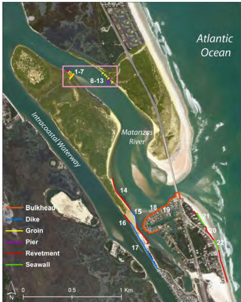
Figure 2.2 Inventory of Coastal Structures in Fort Matanzas Area (NPS, 2013)
