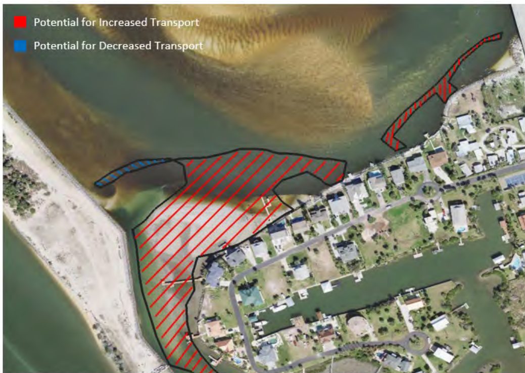
Figure 4.39 Scenario 3 (SHR Deepened to -10 ft NAVD88) Effects on Erosion during Flood Flow
